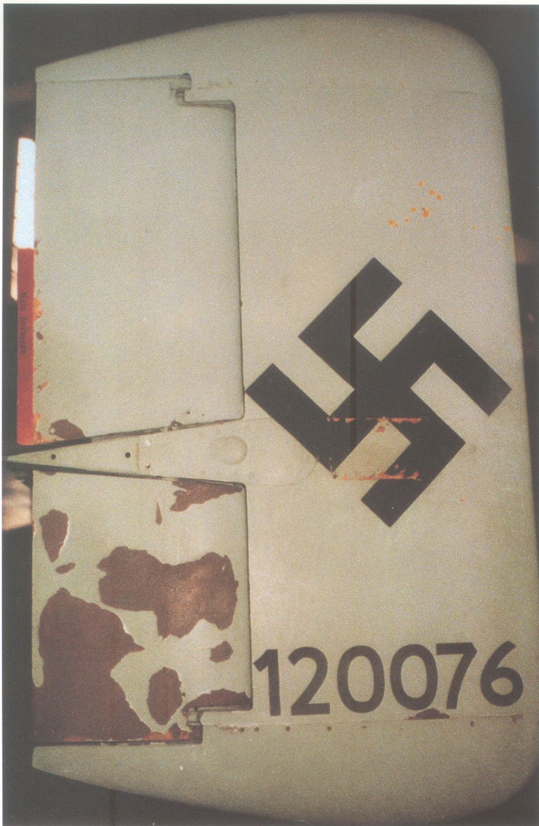
The fin and rudder of a He 162 single-seat day fighter captured by British forces at Leck in northern Germany and later handed over, together with a few more 'Volksjäger', to the French Allies. The Allies had their own jet-propelled designs, and used the He 162s solely to examine Germany's military jet aircraft technology.
